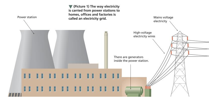
**MAINS** ELECTRICITY is made, or generated, in a power station (Picture 1).
