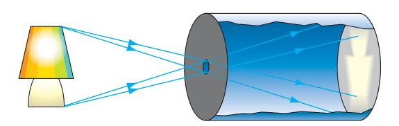
▶ (Picture 5) To get a bright image that is also in focus, you need to use a lens instead of a pinhole.
