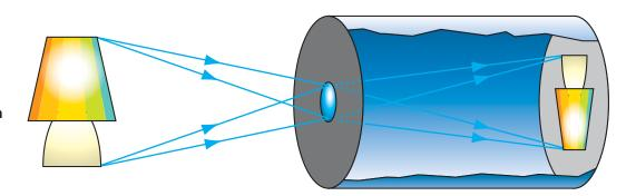
If you hold the pinhole camera to a lamp, for example, you will see an image of the lamp on the tracing paper screen. But the really strange thing is that the image of the lamp will be upside down and back to front (Picture 3).
