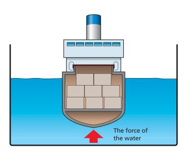
overall, less dense than water. In a similar way, a real ship made of steel is, overall, still able to float (Picture 3).
