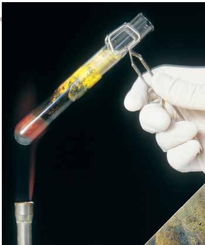
▲► (Picture 2) Permanent change. If you mix iron filings with powdered sulphur, and then heat them with a very high heat, the sulphur and iron combine. A new substance has been made. You cannot separate the iron and sulphur in this new substance. This is an example of an irreversible change.
