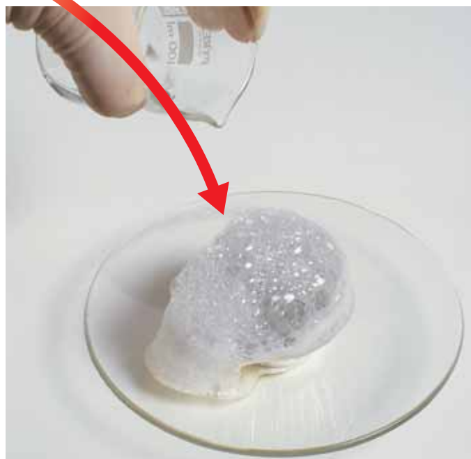
▼ (Picture 3) The fizzing that occurs when caustic soda is poured into the holder.
