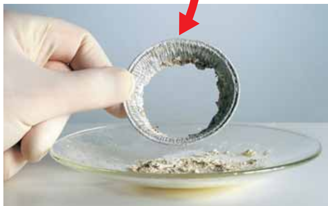
▼ (Picture 4) Within a few seconds the bottom of the holder has been eaten away.
