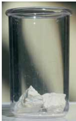
▲ (Picture 1) When vinegar is added to a piece of chalk fizzing occurs. The gas is carbon dioxide.
