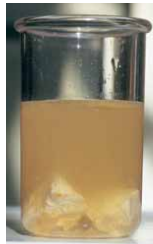
▲ (Picture 1) When vinegar is added to a piece of chalk fizzing occurs. The gas is carbon dioxide.
