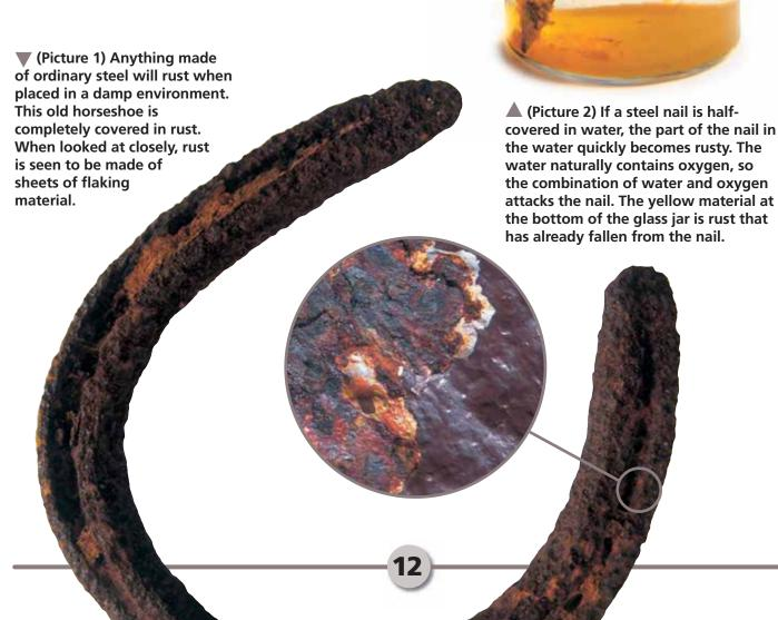
Iron or steel will not combine with oxygen if the air is dry, however. This is why nails stay bright and shiny indoors. But as soon as water is present and the air gets damp, both metals rust quickly (Picture 2).
