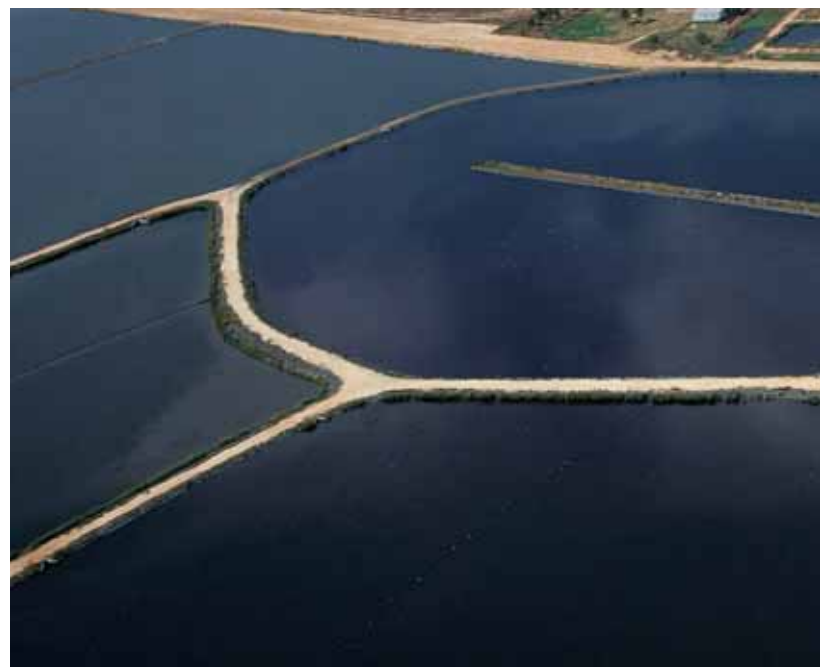
► (Picture 2) A water treatment plant uses big lakes to allow suspended substances to settle out, then the water is filtered through large circular beds of sand. Only then are the dissolved substances treated.
