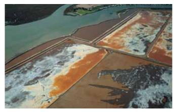
(Pictures 2 and 3) The sea contains huge amounts of salt. People collect this sea salt by allowing the sea water to evaporate in lagoons. These are called salt pans. Because water evaporates faster when the water and the air are warm, most salt pans are found in places with warm climates, not cold ones.
