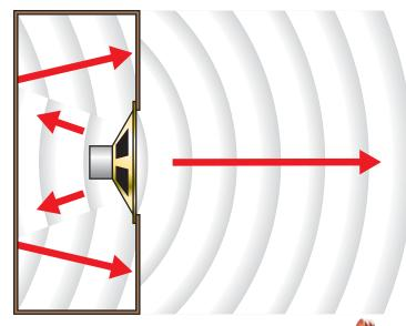
(Picture 2) A loudspeaker sends out waves in front and behind. The cone of the speaker cannot vibrate well enough on its own, so the sound is quiet and 'tinny'. If the speaker is placed in a box, the box also vibrates. Because the box is bigger, the sound is louder and the box is better able to send out low notes. The sounds behind the loudspeaker bounce around inside the box and, if the design of the cabinet is right, they can add even more to the sound.
