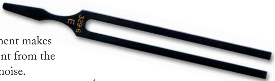
▲ (Picture 1) A tuning fork vibrates to produce a single, pure sound.
