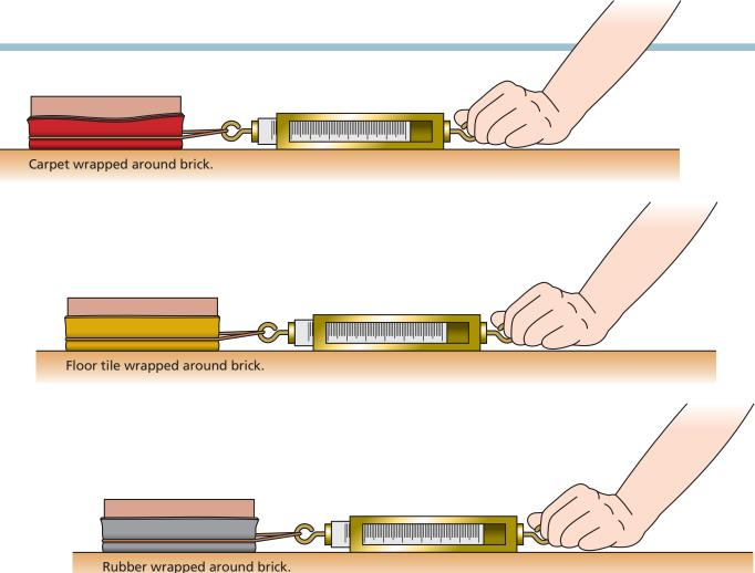
(Picture 2) You can test the friction of various materials by wrapping them around a brick. Always drag the materials over the same surface and at the same speed.
