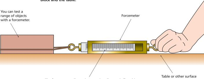
The forcemeter tells you how much pull or push (force) is needed to overcome friction. Watch the scale as you try to pull the block. The scale shows the force you are using. The block will only move when you pull with more force than the friction.
