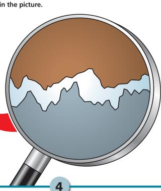
(Picture 2) When you look at surfaces very closely, you find they have bumps and troughs that interlock. This is what keeps most surfaces from gliding over each other easily.
