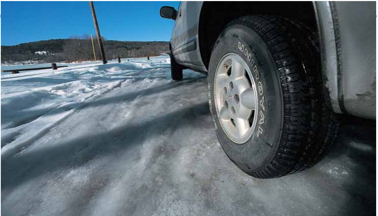
▲ (Picture 3) Cars will slide on ice, not just because it is smooth, but because a film of water forms under each tyre.
