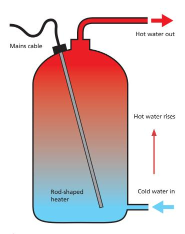
(Picture 3) In a hot water tank, hot water is taken from the top, and more cold water flows in from below. This means that you draw off all of the hot water before you draw off any cold.
