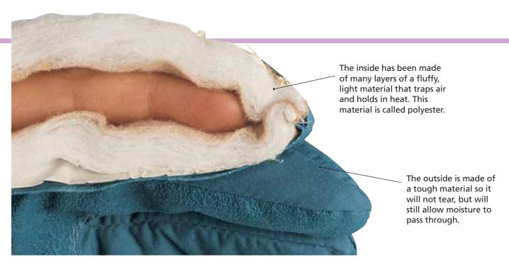
▲ (Picture 2) This cross-section of a ski-glove shows how many layers of fibre are used to trap air and insulate the fingers.
