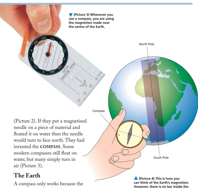
A compass only works because the magnetism in the compass needle is affected by magnetism in the Earth. Scientists have found that the centre of the Earth is made from iron, and this is what makes the Earth into a giant magnet. It works just as though there was a giant bar magnet inside (Picture 4).
