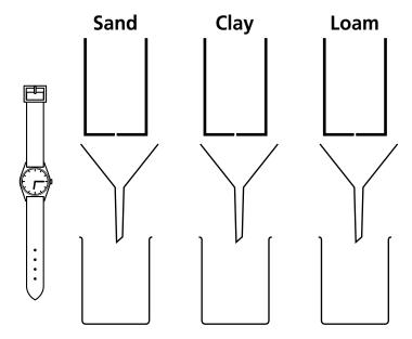
**Q1**. The equipment in the diagram is set up to compare how water passes through sand, clay and loam. The pots each have the same sized draining holes. Name three other things that must be done to make the test fair.
