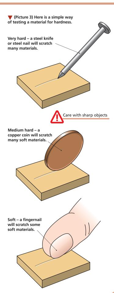
You can compare the hardness of all sorts of materials using just a steel knife or steel nail, a copper coin and your fingernail (Picture 3).
