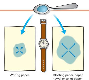
(Picture 4) This is how to compare the absorbency of different papers. Make sure they are all the same size and thickness, pour exactly the same amount of water onto each paper, then leave them for the same amount of time before checking to see how much of each paper is wet.
