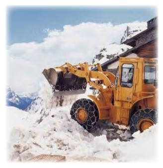
This snow-clearing machine has chains on its tyres to give it better grip.
