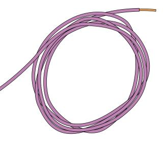
Materials are useful if we can change their shape. We can do this by cutting them, or filing. But it is very useful if we can change the shape of something just by pushing or pulling. Some metals, such as copper, bend easily.
